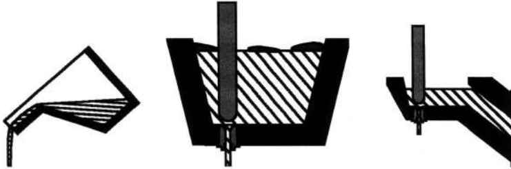
Fig. 3: Tilting ladle, stopper ladle, pressurized pouring system
